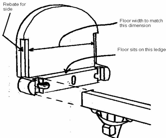
5. Check that the corners of the styrene floor are square, and if necessary, reduce the length with glass-paper to exactly 106mm. The floor is supplied at a nominal 50mm width. Check that the width is the same as the inside of the rebates on the resin end castings. If resin shrinkage has occurred, it may be necessary to trim the floor carefully until it is the same width.
