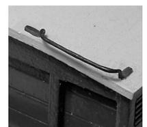
57. Cut side luggage rails from 0.5mm rod, thread on knobs, and glue knobs (called 'props' in an SER specification) into roof holes with superglue. Cut end luggage rails from 0.5mm rod or wire, and curve gently through thumb & forefinger. Thread on knobs, push into roof holes. Line up one end of rail with outer knob, then trim other end to fit against the opposite knob. Solder ends of rod to outer knobs.
