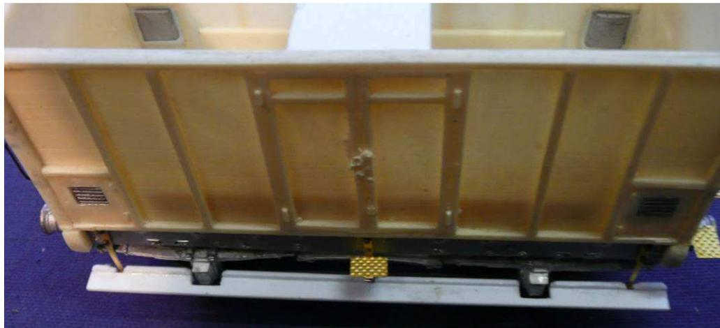
38. Offer the running boards to the carriage and file to fit around the axleboxes as in the diagram and photo
