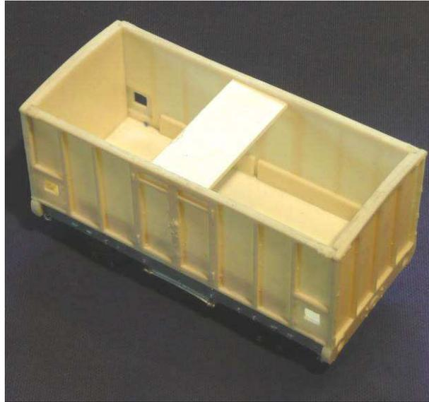
6. When satisfied, glue the floor into one end, then glue one side to end and floor, checking that top strapping detail lines up. Hold the body down on a truly flat surface (preferably plate glass) until the glue has set.
