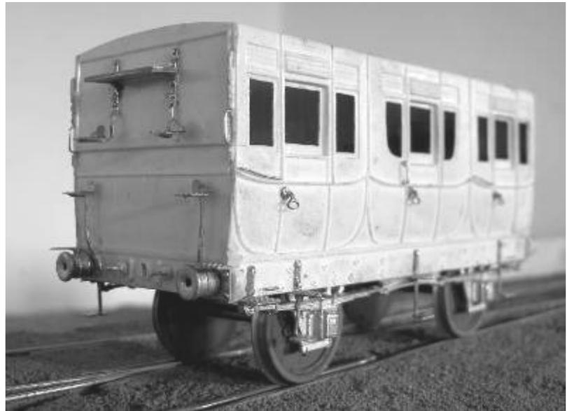
36. Bend end and solebar grab-handles from 26 SWG brass wire and superglue into the holes drilled earlier.
